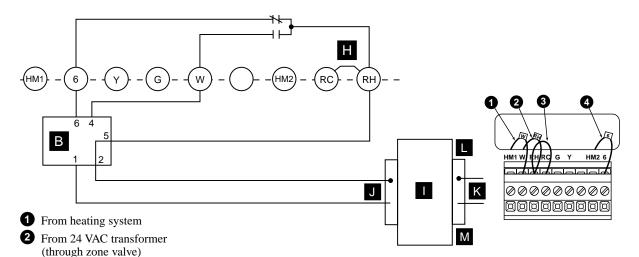
NOTE: Thermostat must have batteries installed. NOTE: Ensure that RED RH/RC jumper wire (provided with thermostat) is connected between thermostat's RH and RC terminals for proper operation with this system.
